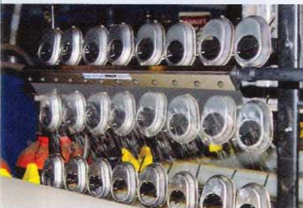
A Model 110024SS 24" (610mm) Stainless Steel Super Air Knife dries bolt covers exiting an electro-polishing tank.
