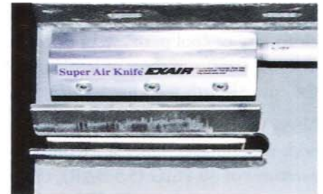
High volume airflow from a Model 110006 6" (152mm) Super Air Knife keeps linear induction motors on an indoor roller coaster from overheating.
