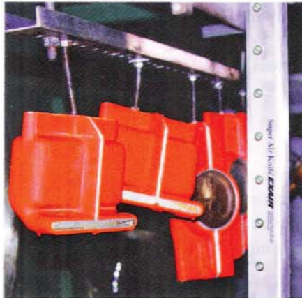
A Model 110018 18" (457mm) Super Air Knife cools molten plastic following dip molding.
