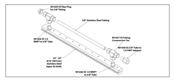
Pipe thread sealant should be applied to 901656 inlet threads (small packet included). Avoid getting the sealant on the inside diameter of the fitting so it does not enter into the Super Air Knife.
