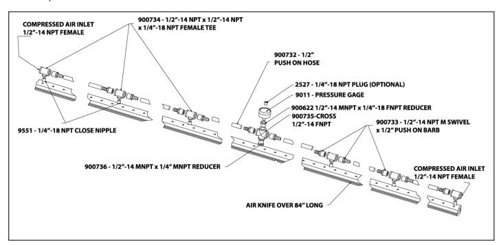
Pipe thread sealant should be applied to all threads (small packet included). Avoid the inside diameter of the fitting so it does not enter into the Air Knife.
