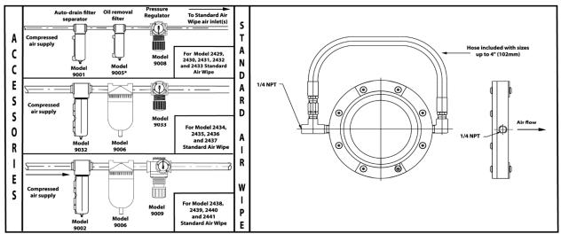
\* Use Model 9006 Oil Removal Filter for Standard Air Wipes that are 3" (76mm) and larger
