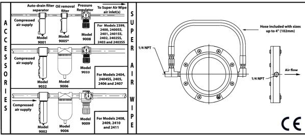
\* Use Model 9006 Oil Removal Filter for Super Air Wipes that are 3" (76mm) and larger
