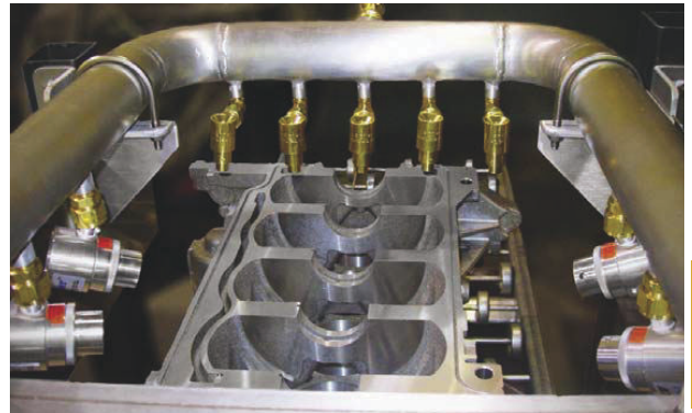
Adjustable Air Amplifiers and High Velocity Air Jets dry an engine block prior to assembly.
