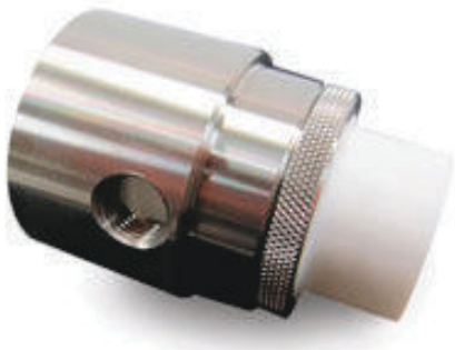
The airflow from this stainless steel Adjustable Air Amplifier with PTFE plug helped pull a sticky material through a process and prevented the material from depositing on the Air Amplifier.
