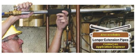
The 3' extension on the Model 1215-3 Super Blast Safety Air Gun helps an operator provide maximum blow off force to remote, tight or difficult to access areas.
