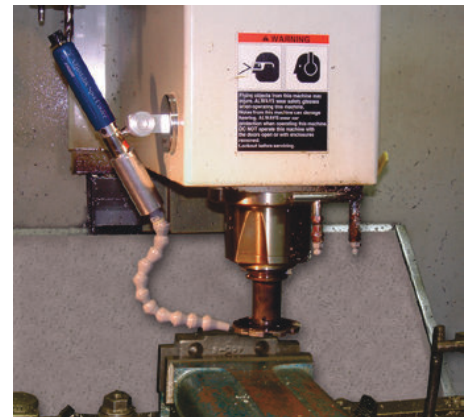
The Adjustable Spot Cooler replaces flood coolant and eliminates hours of cleanup on a cast iron machining operation.
