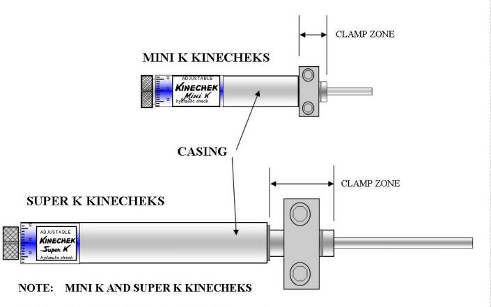
CLAMP BLOCK OR OTHER HOLDING DEVICE MUST FIT WITHIN THE NOTED CLAMPING ZONE OR DAMAGE MAY OCCUR.
